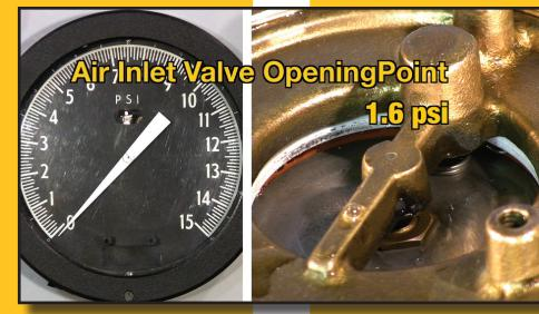
procedures for the reduced pressure principle backflow prevention assembly (RP) using 2 and 3-needle valve gages along with diagnostics.
